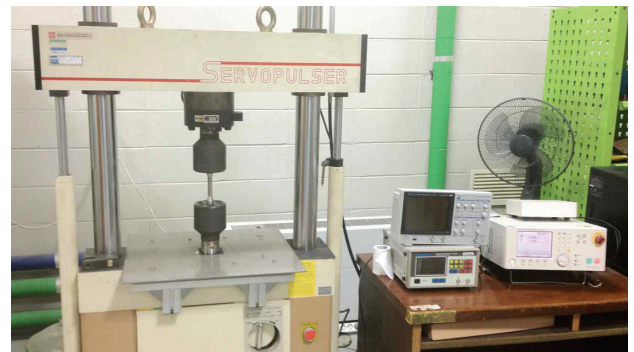
Fig. 1 Fatigue testing machine and Ultrasonic test instrument
