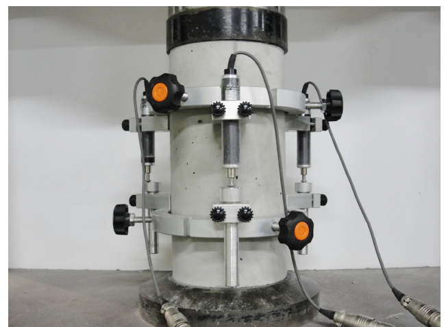
Fig. 3 Set-up for compressive strength test
