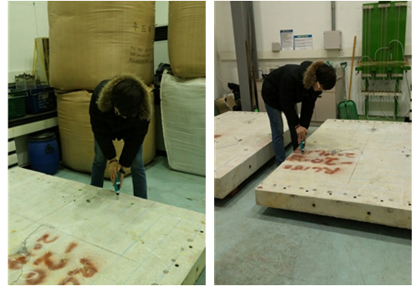
Fig. 6. Rebound hardness test.
