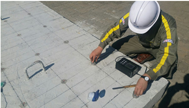
Fig. 5. UPV test in a grid on the concrete slab surface.
