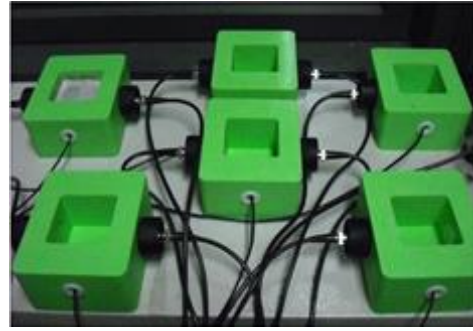
Analysis of mortar on time axis using UC-170, MUX and container
