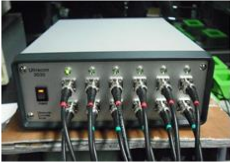
Analysis of mortar on time axis using UC-170, MUX and container
