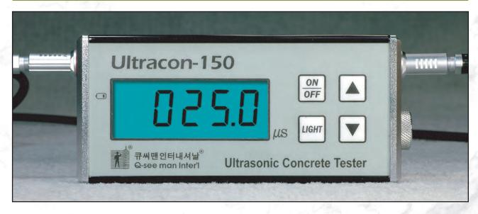
The velocity of ultrasonic wave in concrete is affected by elastic property or strength.
