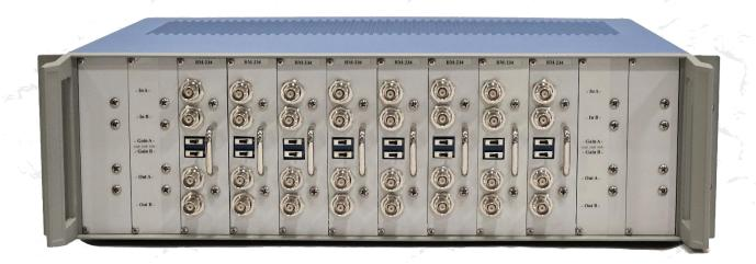
A flexible low noise pre-amplifier system for conditioning small signals. Custom gain, frequency response, and input impedance available by request.
