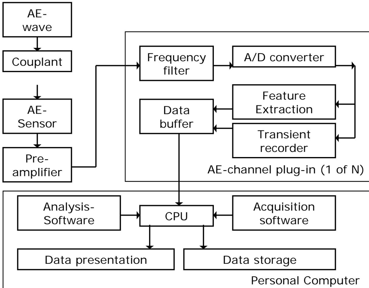
**Figure 8:** The AE measurement chain
