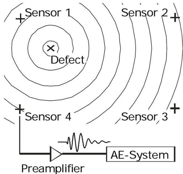
Figure 17: The principle of localization
