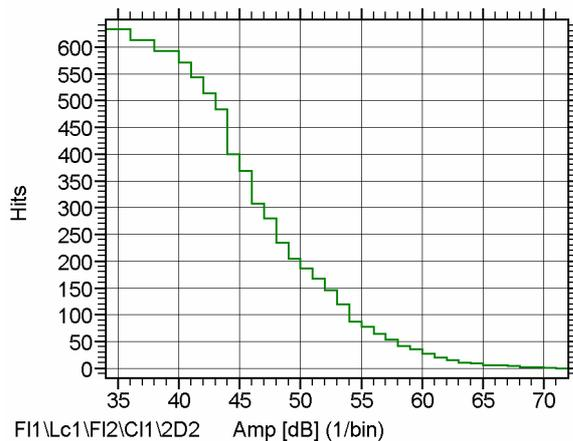
**Figure 29:** Amplitude distribution, cumulative down
