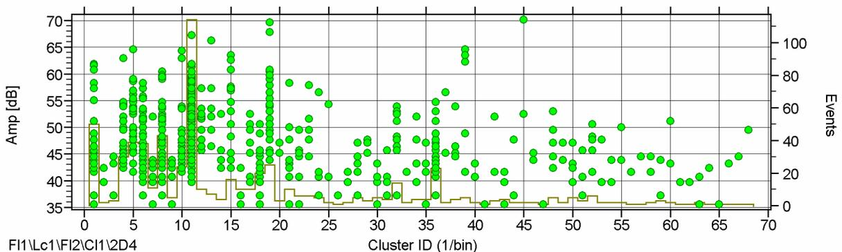
Figure 21: Amplitude and number of event vs. the cluster ID
