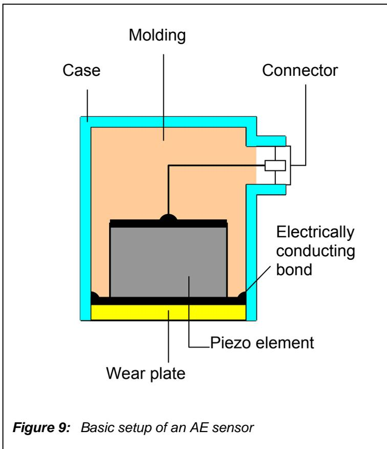
Piezo-electric sensors have proved to be most appropriate for AE testing. They are robust and more sensitive than other sensor techniques, e.g. capacitive, electro-dynamic, or laser-optical sensors.
