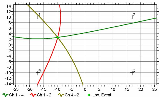
Figure 19: Hyperbola intersection with 3 hit sensors
