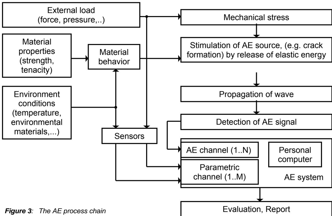
Figure 3: The AE process chain
