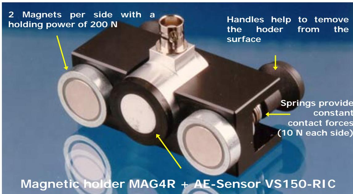
**Figure 12:** Magnetic holder including sensor
