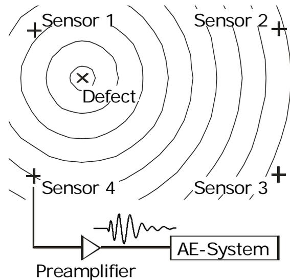
**Figure 2:** Propagation of sound
