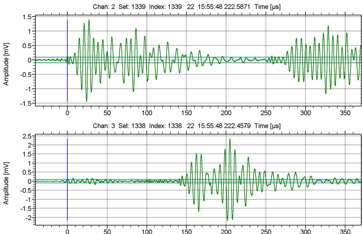
**Figure 23:** Location error caused by the acquisition being triggered by different wave modes. Top: a0, bottom s0
