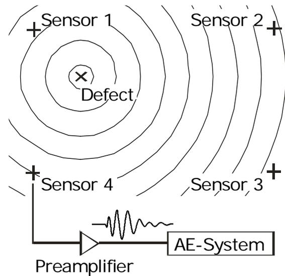
**Figure 2:** Propagation of sound
