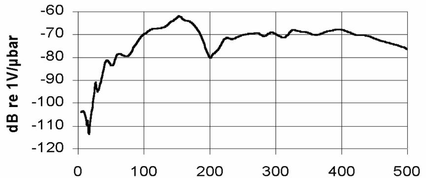
**Figure 11:** Frequency response of a resonant 150 kHz sensor (kHz)
