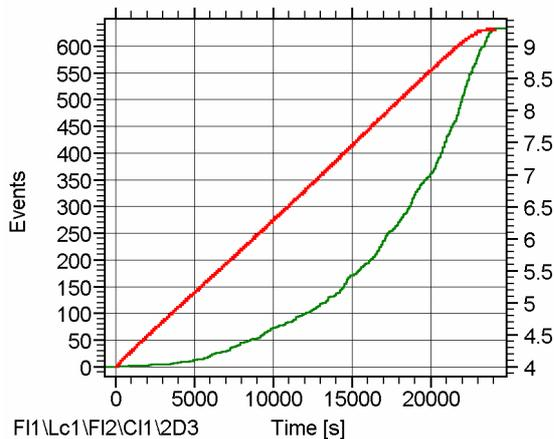
**Figure 25:** Cumulative diagram of the total number of events vs. time incl. superposed curve of linearly increasing pressure
