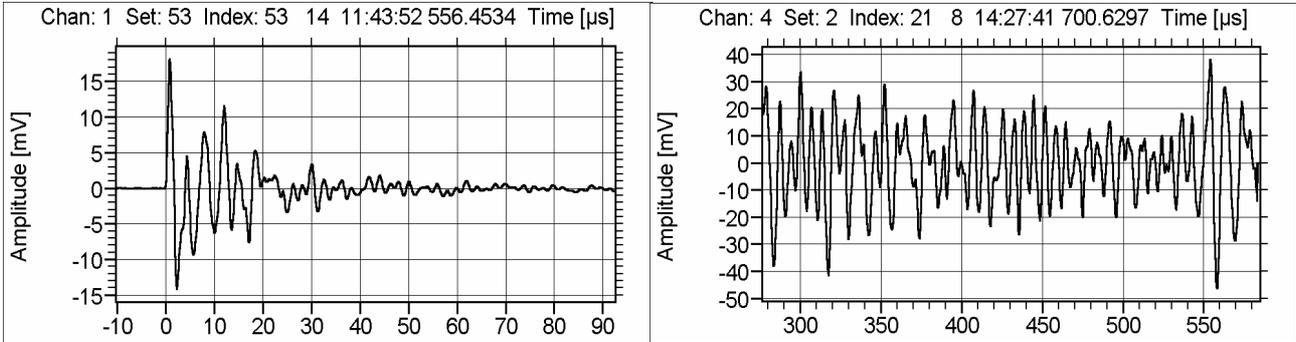
**Figure 4:** Transient (left) and continuous (right) AE signal
