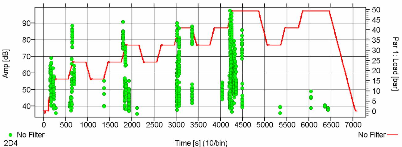
**Figure 28:** Point diagram of the amplitude (intensity) vs. time with superposed pressure curve showing periods of constant and decreasing pressure
