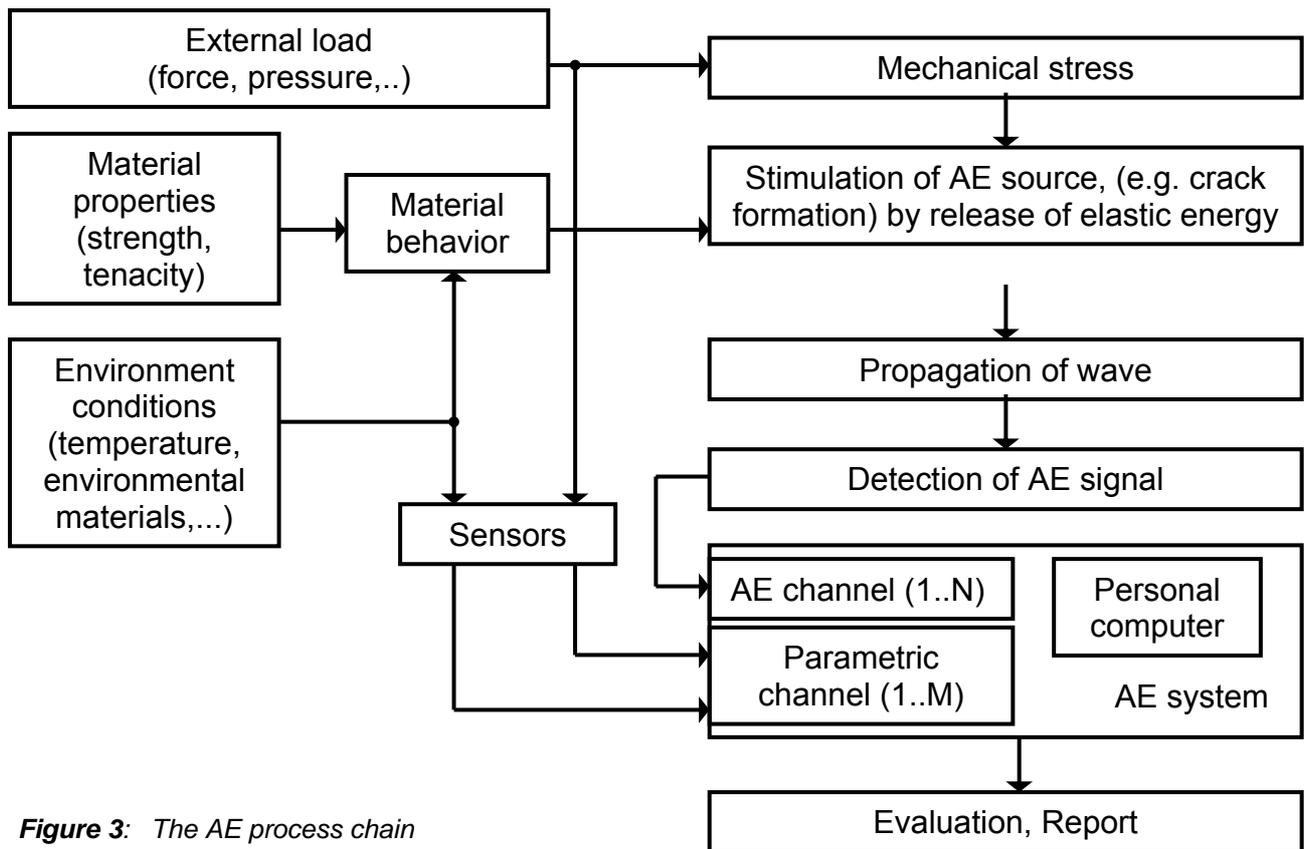
Figure 3: The AE process chain
