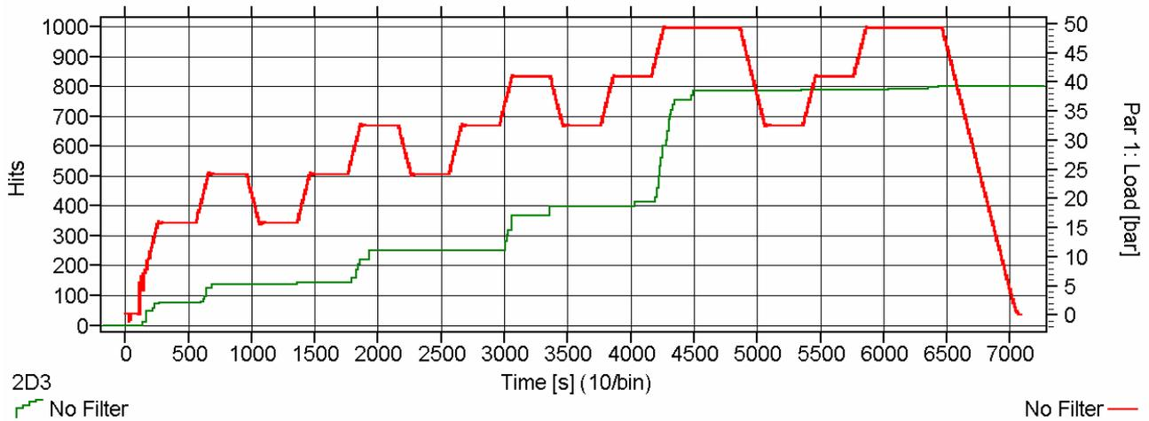
**Figure 27:** Cumulative diagram of the total number of hits (activity) vs. time with superposed pressure curve with periods of constant and decreasing pressure
