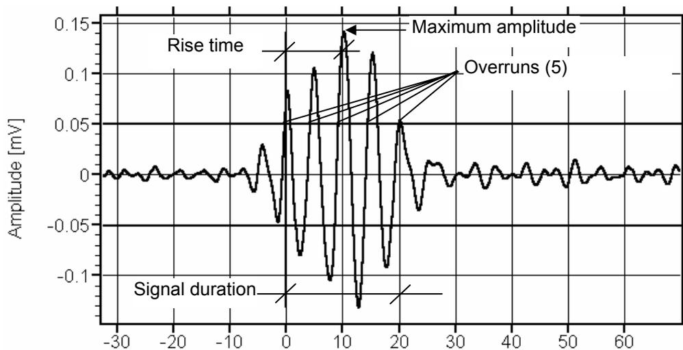
**Figure 6:** Features of transient signals
