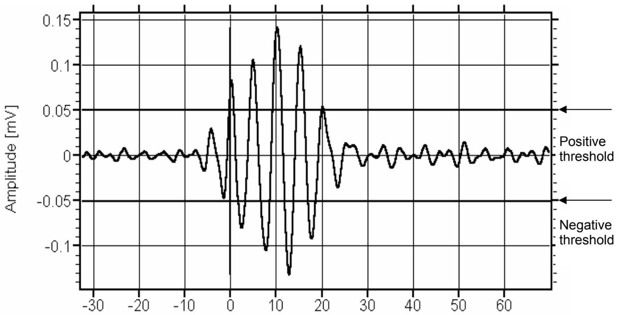
**Figure 5:** Determination of the arrival time. First threshold crossing = arrival time
