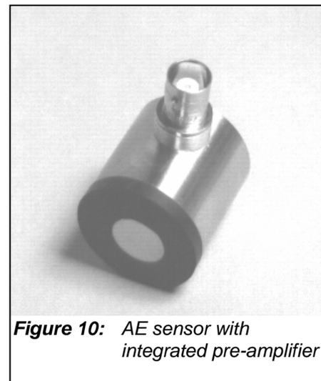
When testing metal vessels for integrity, frequencies between 100 and 300kHz are usually most interesting. The sensors used for this frequency range have a resonance at about 150 kHz and cover
