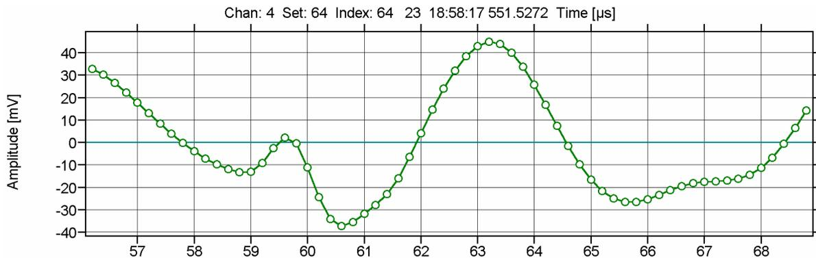
**Figure 14:** Section of the maximum amplitude at 63.2  $\mu\text{s}$ . Bullets correspond to measured values at a sample rate of 5 Msamples/second
