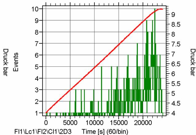
**Figure 26:** Differential plot of the event rate vs. time with intervals of 60 s (with superposed pressure curve)
