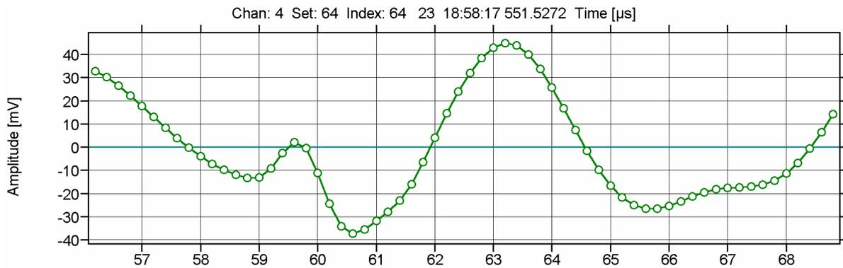
**Figure 14:** Section of the maximum amplitude at 63.2  $\mu$ s. Bullets correspond to measured values at a sample rate of 5 Msamples/second
