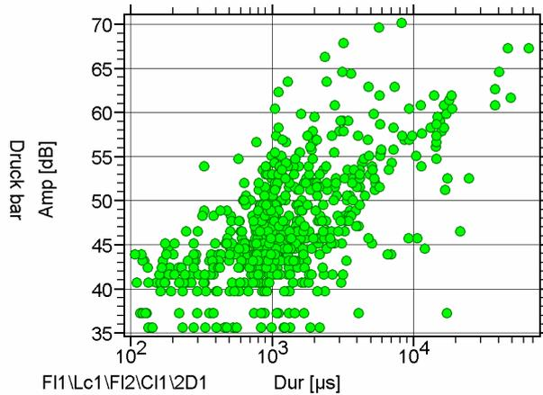
**Figure 32:** Point diagram of the amplitude vs. duration
