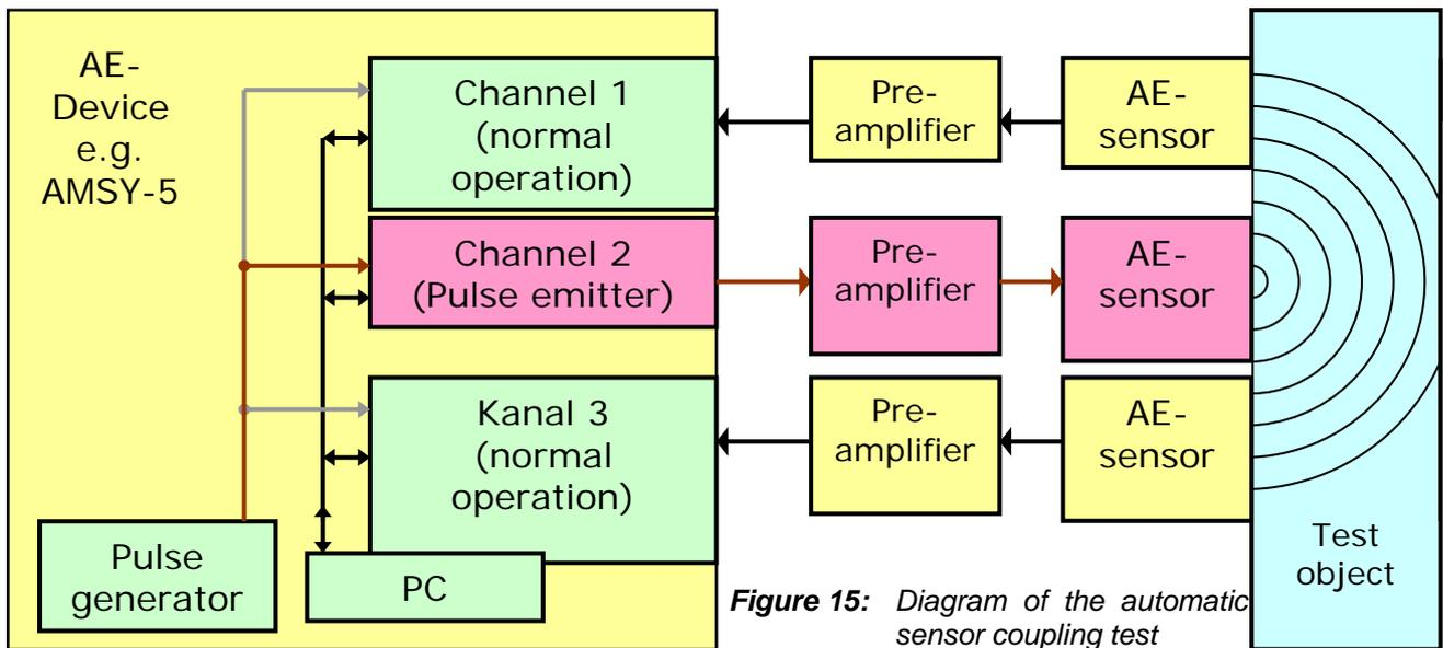
Figure 15: Diagram of the automatic sensor coupling test
