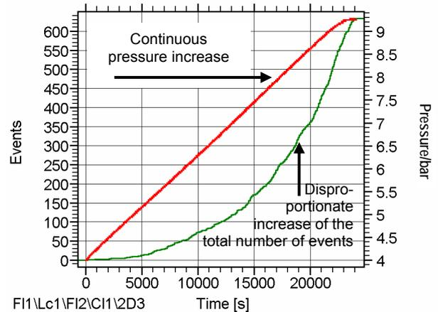
**Figure 7:** Events (left axis) and pressure (right axis) vs. time
