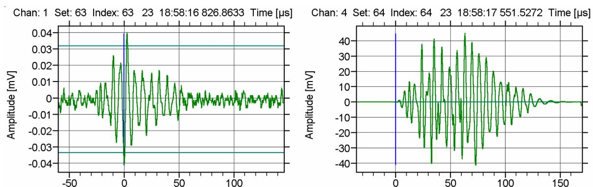
**Figure 13:** AE signal dynamics - bursts with amplitudes of 40µV (left) und 40mV (right)
