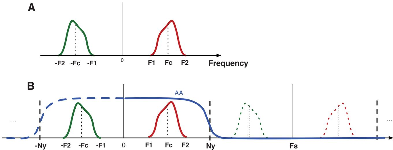
Figure 1. Representation of a signal spectrum, 4x sampling, and the Anti-Alias filter.
