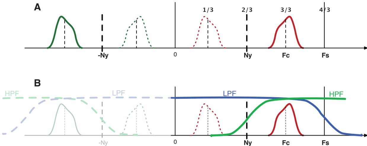
Figure 2. Bandwidth sampling a high frequency signal using a Nyquist limit set below the signal's passband.
