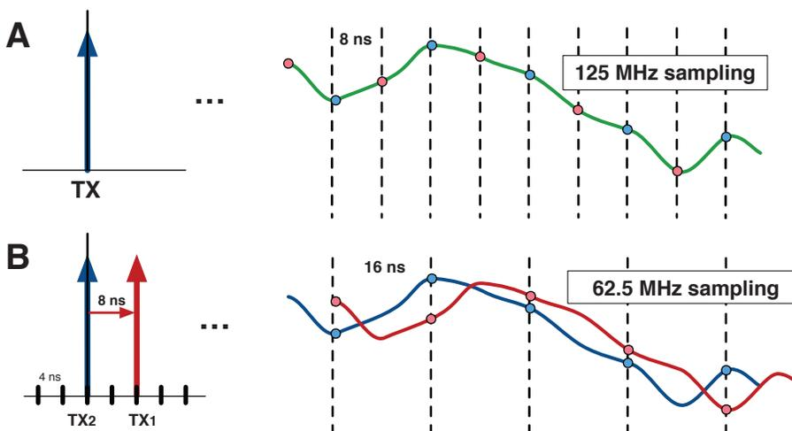
Figure 3. Interleaved sampling using two acquisitions.
