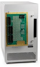
All element signal channels include a breadboard area for surface-mount or through-hole tuning elements, series and parallel positions. Board is normally delivered with zero-ohm series elements in place.
