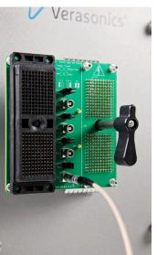
tor, or to acquire data from a single element transducer. This adapter is available now for all Verasonics research systems that use the 260-pin connector.
