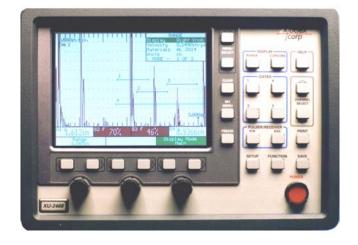
Knob functions are visible without interrupting the waveform display. A pop-up cursor enables quick setup of ultrasonic tests and provides measurements of both thickness and amplitude.
