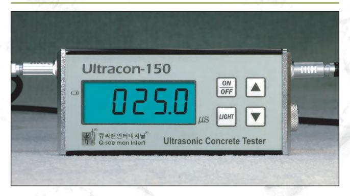
Ultracon-150 measures ultrasonic transit time accurately so it makes possible to evaluate a material or find an elastic property non-destructively to investigate uniformity, cavities, cracks, fire/frost damage, delamination, deterioration and strength in concrete.
